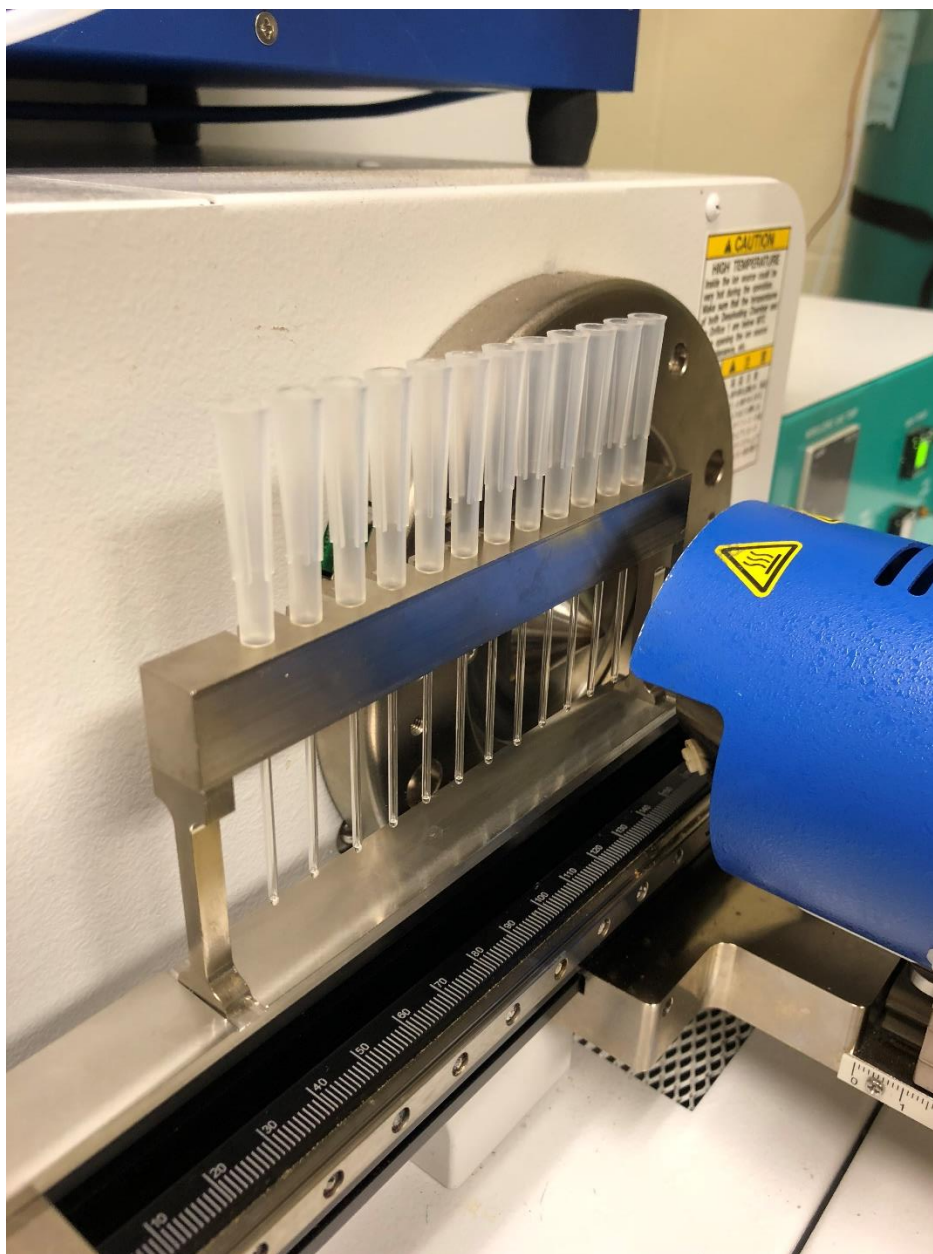
Figure S1. Linear rail system and holder used to position the Dip-it tips with samples between the ion source and the mass spectrometer inlet to introduce samples into the gas stream in order to automate the analysis of calibrators and Kava sample extractions.
